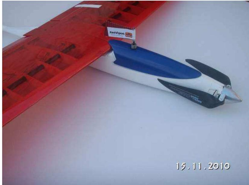
Fig 3 – The transducer fitted in a small electric glider
