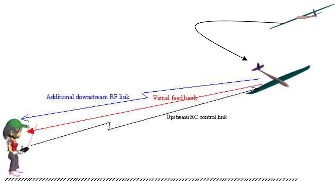
Fig 5 – In flight set-up with HUD
